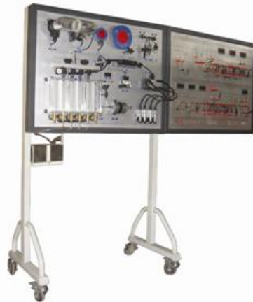
Engine Fuel Oil Supply System Test Bed (For Vw Santana 2000)
