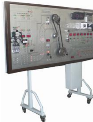
Electric Control System Of Engine Test Bed (For Vw Santana 2000)
