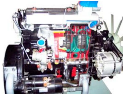
Working Model Of 4 Cylinder 4 Stroke Ci Engine And Gear Box Part Number 0204000004
