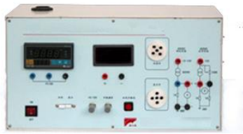
EXPERIMENTAL INSTRUMENT FOR TEMPERATURE SENSOR TEST AND TEMPERATURE CONTROL BY SEMICONDUCTOR REFRIGERATION Part Number 0201010602
