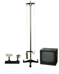
Young's Modulus Of Elasticity Measuring Instrument With CCD Using Stretching Method
