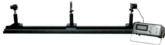
EXPERIMENTAL INSTRUMENT FOR LIGHT INTENSITY DISTRIBUTION OF SINGLE SLIT AND SINGLE THREAD DIFFRACTION
