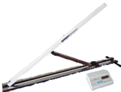
MAGNETIC DAMPING AND COEFFICIENT OF KINETIC FRICTION TESTING LABORATORY APPARATUS Part Number 0201001000
