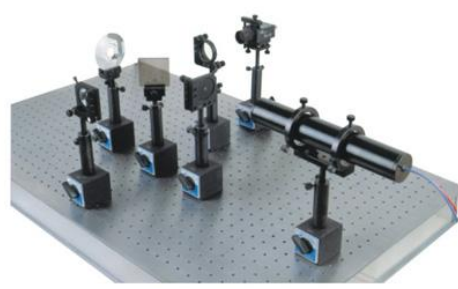
EXPERIMENT INSTALLATION OF ELECTRONIC SPECKLE PATTERN INTERFEROMETRY
