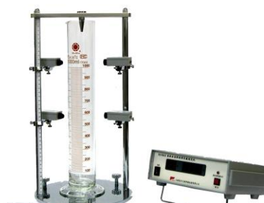
MEASURING INSTRUMENT FOR LIQUID VISCOSITY COEFFICIENT BY THE METHOD OF DROPPING BALL Part Number 0201000700
